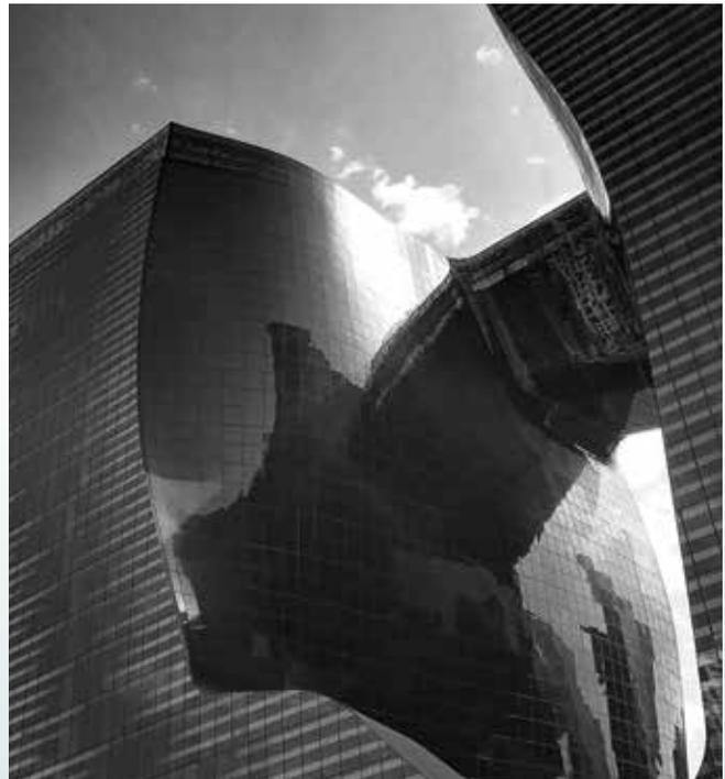
**The Opus, Business Bay, Dubai - Two 20 story towers connected by a bridge, with the inner façades forming a seamless fluid glass surface, resembling melted ice. Undoubtedly one of the most challenging projects in the region, Koltay Façades was using advanced 3D computing technology and building on their earlier experience and research work in freeform glazing methods to deliver this project.**
